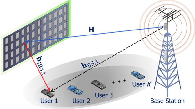
Fig. 1. Illustration of a multi-user IRS-assisted downlink network comprising one BS and  $K$  URLLC users employing finite block length transmissions.  $\mathbf{H}$  is the channel matrix between the BS and the IRS,  $\mathbf{h}_{\text{IRS},1}$  denotes the channel response vector from the IRS to user 1, and  $\mathbf{h}_{\text{BS},1}$  indicates the channel between the BS and user 1.
