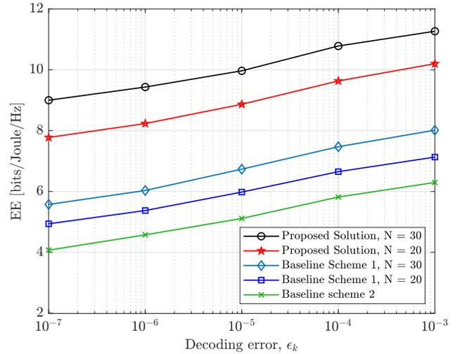
Fig. 2. Impact of tolerable decoding error,  $\epsilon_k$ , on the EE.
