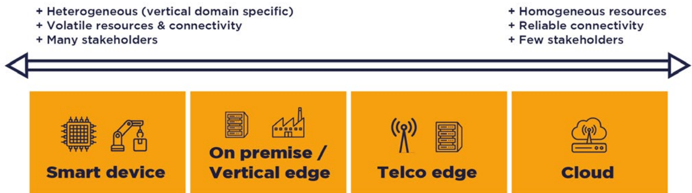
Figure 3-1. Structure of the 6G cloud continuum.
